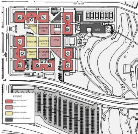
Figure 1.6: LANEY Structural Voluntary Upgrade Analysis
